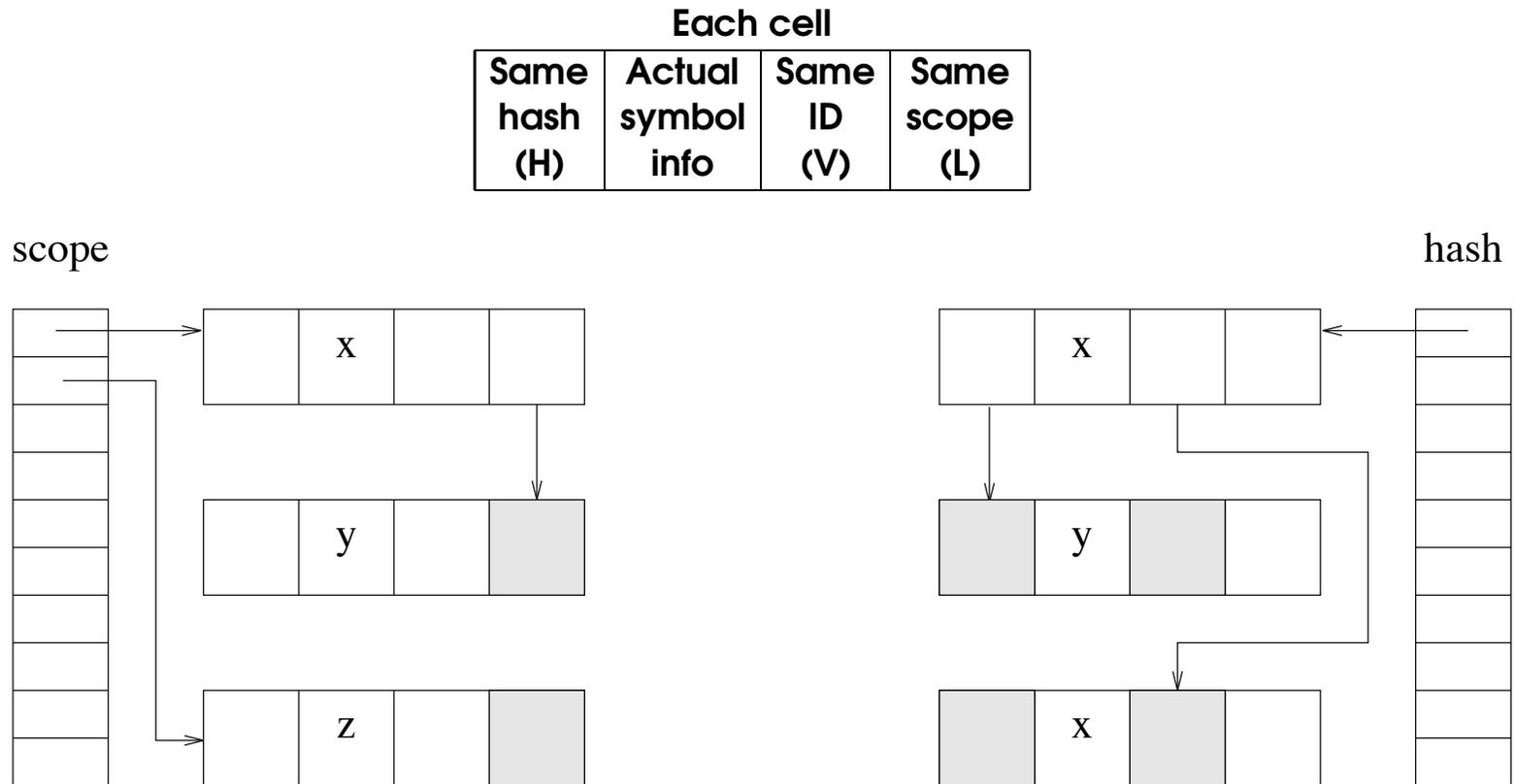
The above scheme implements a stack for each variable  $v$ , where top-of-stack is the currently active instance of  $v$ . Let  $f(v)$  be the hash index for variable  $v$ :
