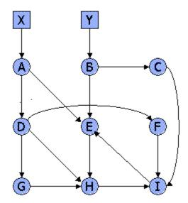
The heap is managed by an incremental algorithm that uses the four lists *Unreached, Unscanned, Scanned,* and *Free,* as in Baker's algorithm. To be specific, the *Unscanned* list is managed as a queue, and when more than one object is to be placed on this list due to the scanning of one object, we do so in alphabetical order. Suppose also that we use write barriers to assure that no reachable object is made garbage. Starting with A and B on the *Unscanned* list, the following events occur:
